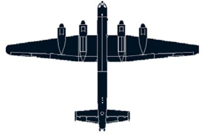
**DAM BUSTERS** The underside of Britain's primary four-engine bomber was almost always painted black because it often flew at night. A "Lanc" could haul seven tons in its long bomb bay.
