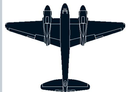
**ATTACKING BERLIN** With a V-shape wing profile and two Merlin engines, the "Mossie" was used by the Royal Air Force as a fighter, bomber, and recon plane. It was made almost entirely of wood.
